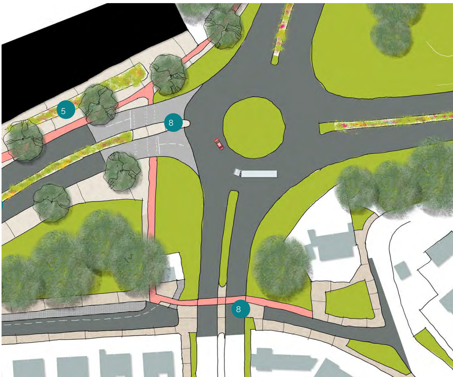
Figure 134. | illustration showing how an approach street environment might be designed to accommodate the mix of goals of allowing through traffic whilst prioritising good movement for pedestrians and cycling
